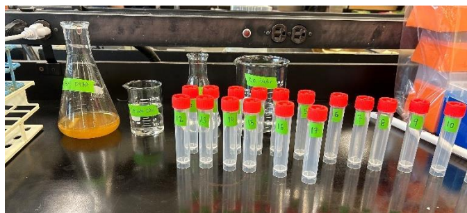
Figure 4-7: Sample preparation for standard curve creation.
