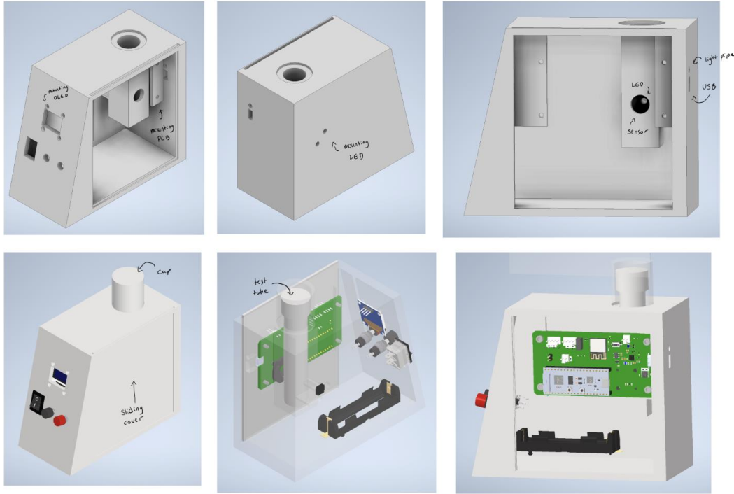
Figure 4-15: Final Mechanical Design
