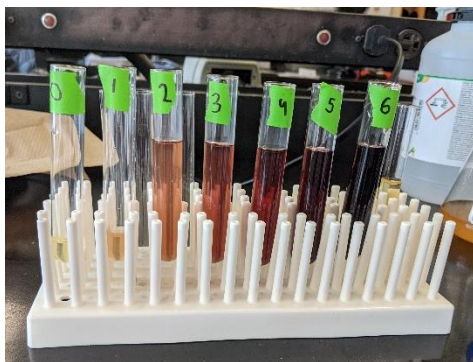
Figure 4-3: Visually distinguishable colour changes following the DNBA reaction with samples containing differing creatinine concentrations.
